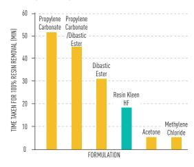
For a procedure in which polyester resin was coated onto aluminium strips, partially cured for (12 hrs) and submerged in a beaker containing the respective formulations, at ambient temperature in the absence of agitation (experiment covered under patent U.S. P. 6.187.108).
